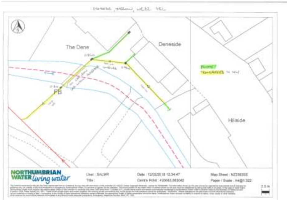
Figure 2: The results of a pipe survey carried out in February by Northumbria Water showing that the sewage from the Dene is carried across the river in a pipe underneath a footbridge (pipe indicated in yellow).
